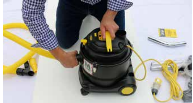
14 Turn clockwise to lock (gently pull to ensure it is locked)
